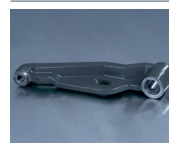
Tensioning arm for pulley manufactured from forged blank, mechanically machined and powder-coated
