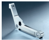
Lever arm as chain attachment for storage systems manufactured from forging blank, mechanically machined, galvanized Additionally assembled to form a module with mounted sliding bearing and plastic cap
