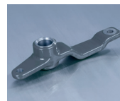
Tensioning arm for pulley manufactured from forged blank, mechanically machined, powder-coated
