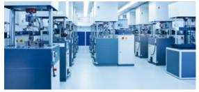
More than **21 pulsers** (worlwide) are available for testing dynamic fatigue strength according to different testing methods
