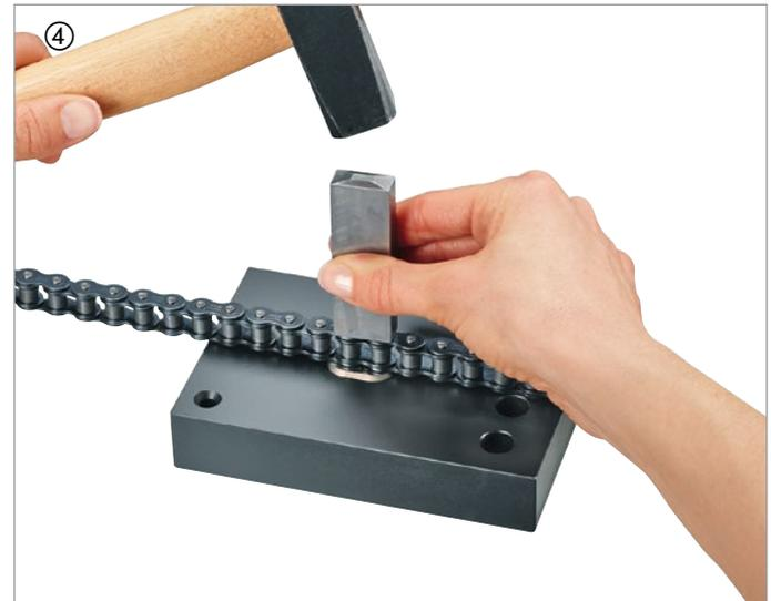
The procedure used is common to both shouldered and parallel bearing pin chains. The new riveting link connects the two inner links. This connecting link is supported by an insert in riveting plate ③.
